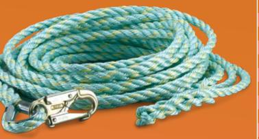
Our Polysteel™ safety lines are manufactured to CSA Z259.2.5. The standard configuration includes a thimble and spliced eye with either a carabiner or snap hook attached at one end and a back splice at the other end. The safety lines can be supplied with alternate CSA Certified hooks attached where required. Please refer to pages 14 - 16 for available hooks and other accessory products.
